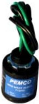
The T1SPD is an easy to install surge protector that meets all applicable electric codes. It is used for 120/240 electrical services and can be used in pairs for 240 V Delta 3 phase and 120/208 Wye 3 phase services. The T1SPD is rated to handle surges 25% higher than the average lightning strike so it will work reliably for years. The T1SPD design prevents failure due to open neutrals or other system disturbances.
