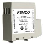
The **PEMCO DRS Series** is a din rail mountable, single pair surge suppression module implementing three-stage hybrid technology. This module addresses overvoltage transients with gas tubes and silicon avalanche components. In addition, sneak currents are mitigated with resettable fuses (PTCs). The PTCs increase resistance several orders of magnitude when overcurrents exceed safe levels. A normal state
