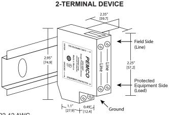
Wire Size Range = 22-12 AWG Terminal Torque Rating = 0.8 Nm (7 in-lb)
