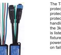
The T4SPD is an easy to install surge protector that is used for lighting system protection as well as control panel protection. The T4SPD is capable of handling a 10kA peak surge current (triple the 3kA expected on wired devices) and is listed for use inside panels and lighting fixtures. LM model does not disconnect power on failure. LMT disconnects power on fail.
