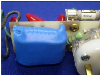
The exclusive X-Coil design (US Patent #7,085,115 B2) prevents surge energy from entering the last stage by blocking and dispersing energy that gets through the first stage. This provides high frequency filtering yet at the same time passes normal power current along without overheating. Similar induction coils with ferrite cores get hot during normal operation from hysteresis losses. The X-Coil advantage is that such losses are small so it does not overheat.
